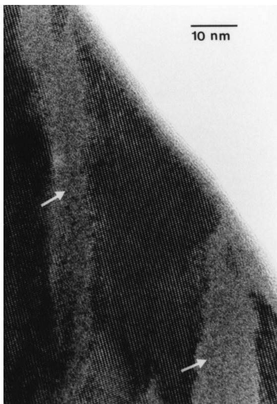
FIG. 3. HREM image of the (010) plane of Gd_3(BO_3)_2F_3 (white arrows point out amorphous domains damaged under the electron beam).
